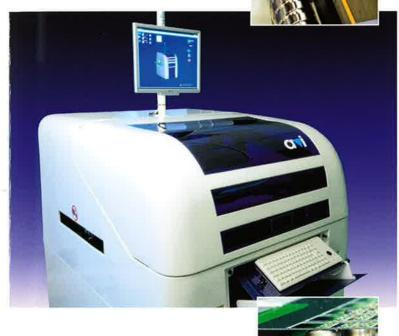
Automatic rail width adjust is standard to aid quick changeovers in a high mix manufacturing environment.
